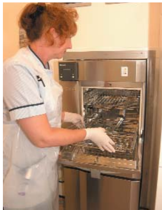
Spotless: after the 30-minute cycle equipment is unloaded in the 'clean' room prior to autoclaving
